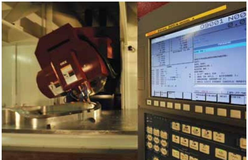
programs postprocessed for the tool-rotation machine could not be used on the new table-rotation machine. To move work readily from one machine to the other, Desemco's programming staff would have to acquire the appropriate post-processor for the second machine and apply that to the original tool path data generated in the five-axis programming software from Mastercam
