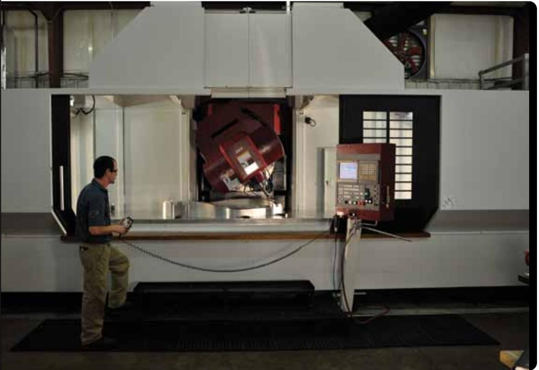
A five-axis machine with an extra-long table provides the flexibility to handle either one large part in a single setup or several smaller pieces set up on different sections of the table. The rotary axes of this machine are in the spindle head, as shown at right.
