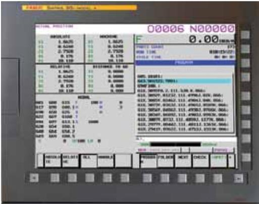
developed by the company to enhance five-axis machining productivity. The vector programming option complemented other advanced CNC functions such as automatic tool center point (TCP) control, tool position control (TPC), nano-smoothing and high speed smooth TCP. All of these functions apply sophisticated software routines to adjust the position and orientation of the cutting tool for smoother, faster machining.
